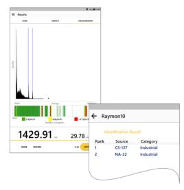
Once a spectrum has been recorded, fully automated radionuclide identification can be performed against a library of commonly encountered radionuclides to ANSI N42.48 standards.
