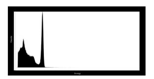
The Nal Probe produces defined spectral peaks for reliable spectral analysis on the RayMon
