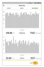
The measurement screen allows the user to view count data for Alpha and Beta radiation as a bar chart meaning changes in count rate can be easily visualised.
