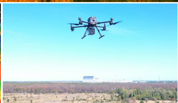
Drone flying over the Red Forrest: Each survey route is saved as a collection of GPS waypoints, altitudes and velocities allowing the same survey to be conducted repeatedly to study any change in the distribution of radioactivity over time.
